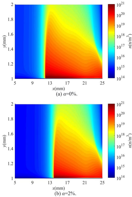
Fig.7 Distribution of density space charge with (a) the ratio of  $H_2O$   $\alpha=0\%$  and (b) the ratio of  $H_2O$   $\alpha=2\%$  when  $t = 12$  ns.
