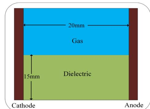
Fig.1 Air-dielectric discharge model with uniform electric field
