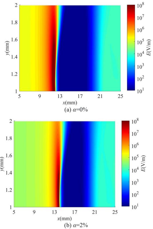
Fig.8 Distribution of strength of electric field with (a) the ratio of  $H_2O$   $\alpha=0\%$  and (b) the ratio of  $H_2O$   $\alpha=2\%$  when  $t = 12$  ns.
